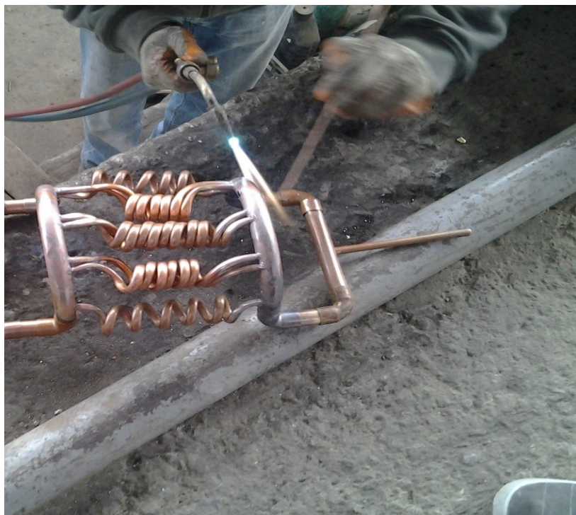
Figure 4.2 Soldering process for the heat exchanger
